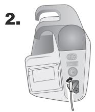
Figure 9-1 Connecting the Sampling Line Connector to the  ${\rm CO_2}$  Inlet Port
