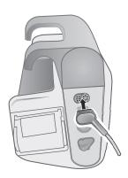
Figure 6-3 Connecting ECG Cable to Propaq MD Unit
