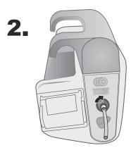
Figure 8-2 Attaching Single Lumen Hose to the Propaq MD Unit
