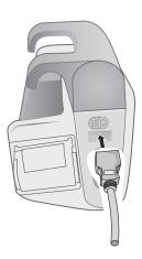
Figure 10-3 Connecting the SpO<sub>2</sub> Sensor to the Propaq MD Unit
