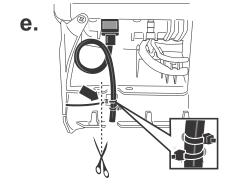
Plug in connector and secure cable.
