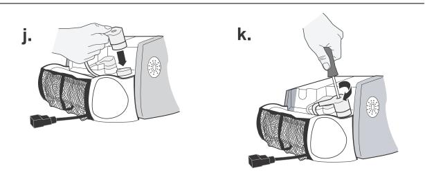
Connect cabling and tighten hardware.
