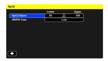
Figure 9-4 SpO<sub>2</sub> Parameter Control Menu
