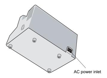
Figure 2-2 SurePower Single Bay Charger Bottom View
