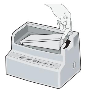
...and then lift the battery out of the charging bay.
