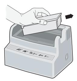
**Note:** If the **Fault** LED is on when you remove the battery pack, the charger beeps to alert you that there has detected a *charging fault*. Do not use this battery pack in a defibrillator or monitor until you have confirmed the nature of the charging fault (for more information, see *Troubleshooting Charging Faults* later in this chapter.
