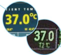
*Patient temperature displayed on both patient monitor and the IVTM System while using only one temperature probe.*
