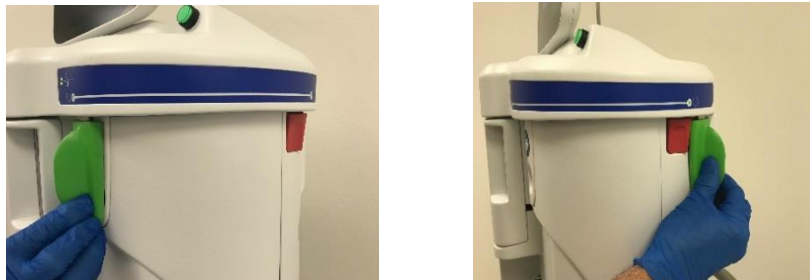
Figure 6. Energizing the DownStream® System Console
