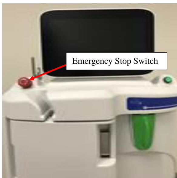
Figure 24. Emergency Stop Switch
